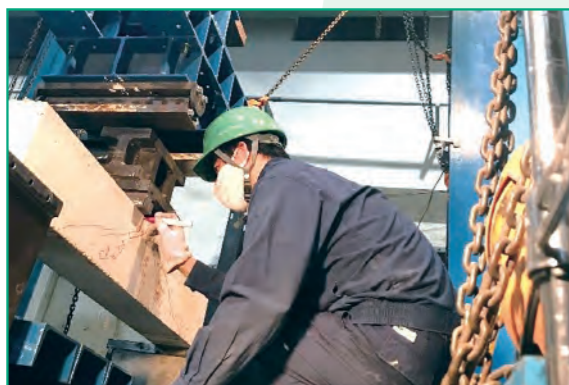
50t load-test apparatus for studying the mechanical properties of reinforced concrete
